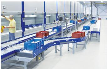
For quick order picking and consolidation of orders, work zones can be easily connected via conveyor systems. Items are delivered automatically to the access opening, picked and then placed into shipping containers on the conveyor. As orders are completed, the containers can be directly routed to shipping via conveyor for a fast and trouble-free operation.
