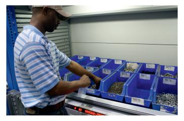
To improve operator productivity, throughput and accuracy levels, Kardex Remstar offers several integrated pick-to-light technologies. Machines can be equipped with TIC (transaction indicator centers), light pointers and confirmation bars to pinpoint the exact location of the transaction required.
